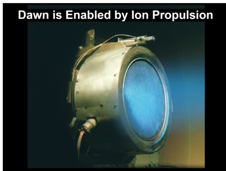
Figure 1. Ion thruster used by the Dawn spacecraft
