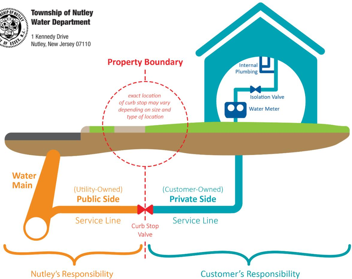
Homes with lead service lines are typically the most significant source of lead in the water. Lead pipes are more likely to be found in older cities and older homes. The homes without lead service lines can also be problematic; as lead can leach from brass or chrome-plated brass faucets and plumbing with lead solder.
