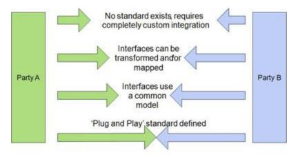
As an illustration, the flash drive in your pocket is a plug-and-play device. It conforms to the USB specification as a specific type of USB device, which is recognized by the operating system to have specific properties and behavior. If the flash drive does not conform to these specifications (or if the correct device driver is not installed in the operating system) then plug-and-play becomes plug-and-*pray* or plug-and-*slay* (as in urge to kill).
